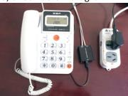
LED light turn on red when connected to power supply, the recorder begins to recording the voice when pick up Setting Date and Time: telephone headset, LED light will flashing | Connect it to computer via USB cable, open one time per second.
