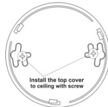
Install the top cover to ceiling with screw, please check the direction.
