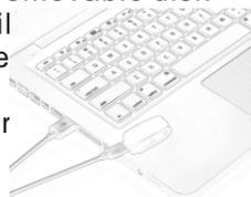
To disconnect, click “safely remove device” from your computer and unplug the USB.
